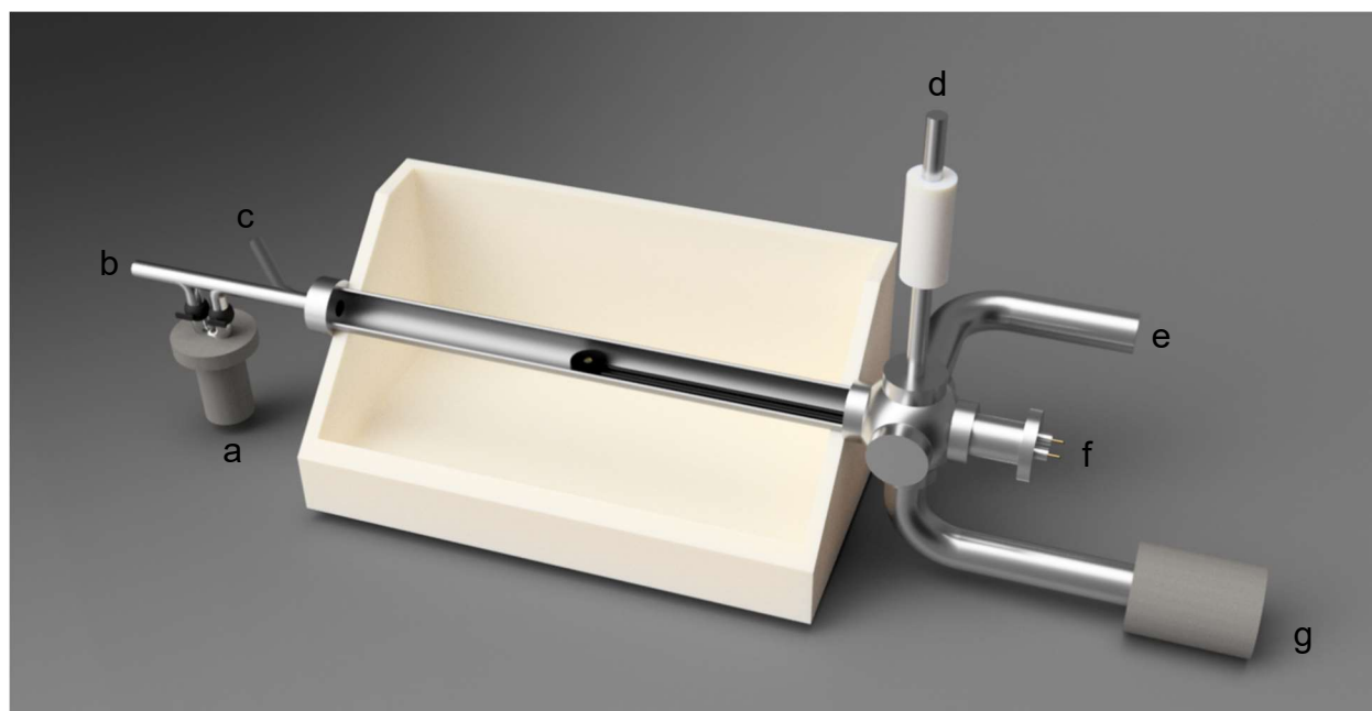
Figure 14. Diagram of the ALD tool used equipped with a 6.985 cm inner diameter and 91.44 cm long stainless-steel furnace tube. With (a) being a steel cylindrical ball valve bubbler, (b) is the carrier gas inlet and (c) is the secondary precursor inlet (which was used for trimethyl aluminum) all equipped with ALD valves from Swagelok. (d) is a Baraton capacitance manometer, (e) connects the system to a liquid nitrogen trap followed by a roughing pump, (f) is the QCM component which extends into the center of the ALD chamber and (g) is a mass spectrometer.
